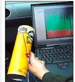
Pringles tube works as an antenna
